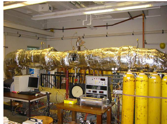
Fig. 20. Insulated closed-circuit wind tunnel with the secondary flow injection system.
